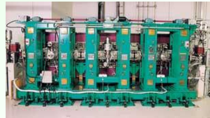
In-vacuum type NdFeB magnet undulator
