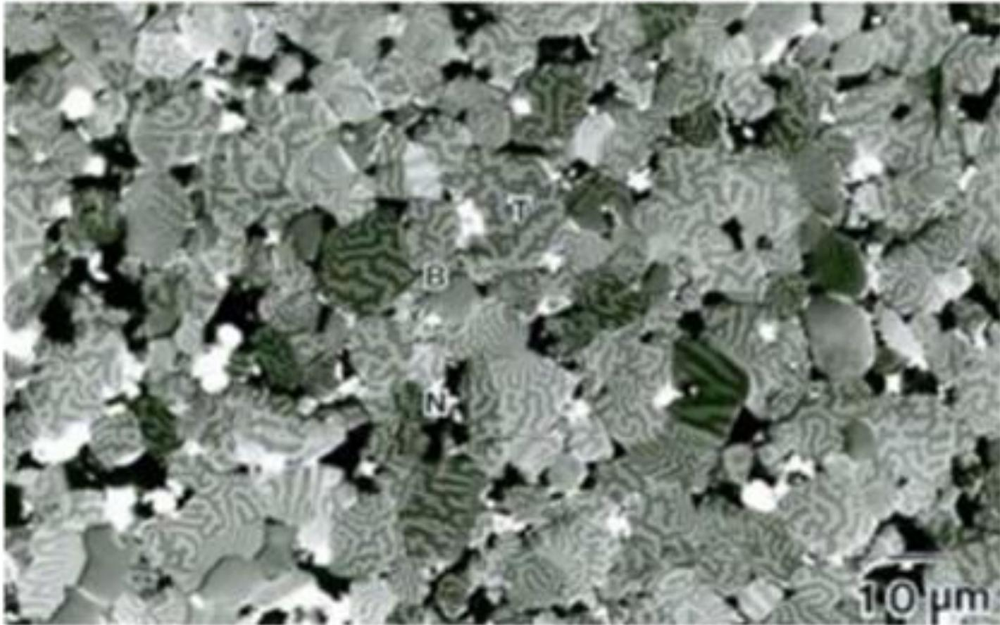
$\text{Nd}_{15}\text{Fe}_{77}\text{B}_8$ 磁石 消磁状態 (c面)
